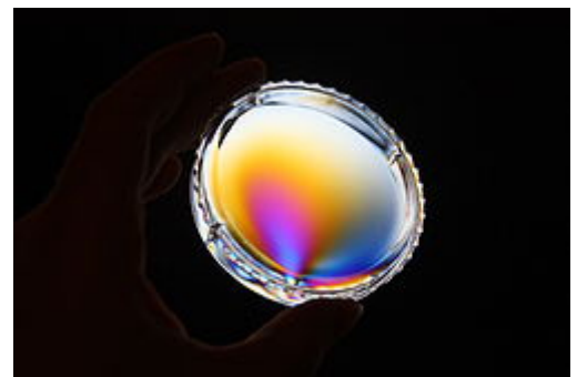
Color pattern of a plastic box showing stress-induced birefringence when placed in between two crossed polarizers.
